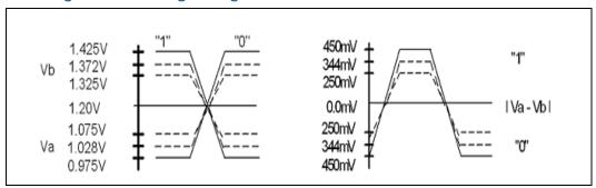
1's and 0's are represented the differential voltage between the pair of signals. As shown in the Figure 15 a serial pattern of 1100011 represents one cycle of the clock.
