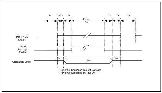
NOTE: Support for programming parameters TX and T1 through T5 via SW is provided.
