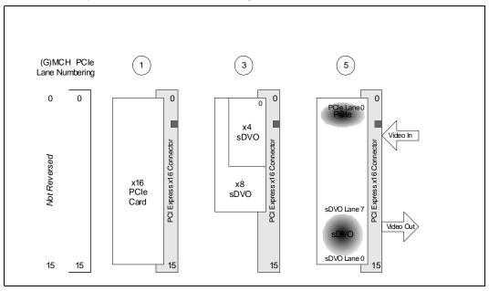
Figure 11. SDVO/PCI Express Reversed Configurations
