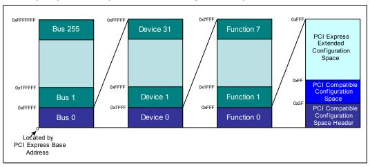
As with PCI devices, each device is selected based on decoded address information that is provided as a part of the address portion of Configuration Request packets. A PCI Express device will decode all address information fields (bus, device, function and extended address numbers) to provide access to the correct register.
