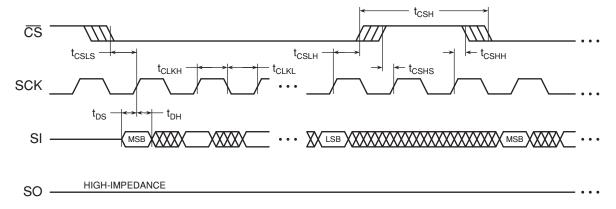
Figure 15-2. Serial Output Timing
