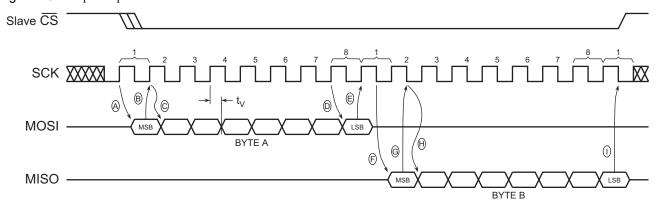
MOSI = Master Out, Slave In MISO = Master In, Slave Out The *Master* is the ASIC/MCU and the *Slave* is the memory device.
