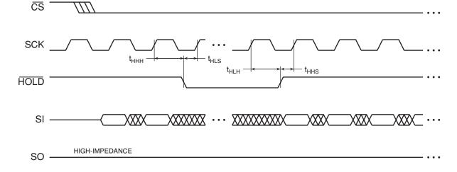
Figure 15-5. HOLD Timing – Serial Output
